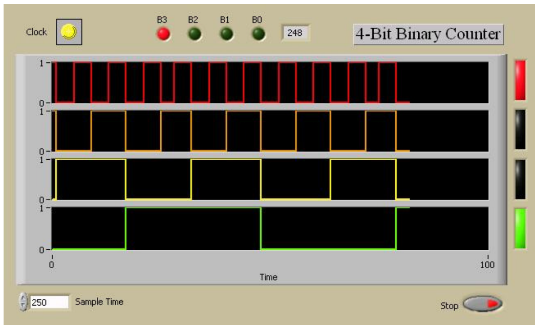
Figure 5.7. Timing Diagram of a four bit Binary Counter
