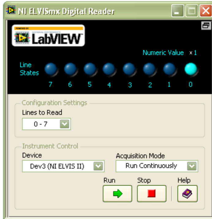
Figure 5.5. Digital Reader reading bit 0, line DIO <0>
