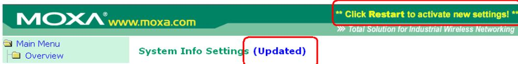
To activate the changes click **Restart** and then **Save and Restart** after you change the settings. About 30 seconds are needed for the AWK-3121 to complete the reboot procedure.
